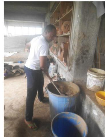
Fig. 8: Mixing clay into slip in a plastic bucket
