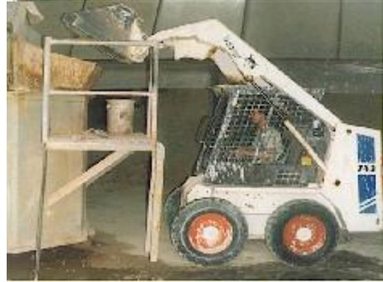
Fig. 2: Crushed clay is then loaded into a blunger where other raw materials and water are added and mixed until a slurry is formed
