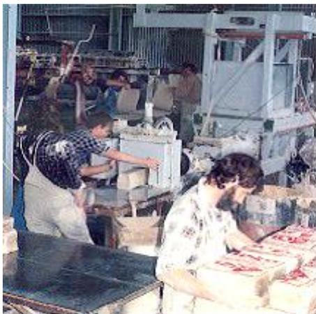
Fig. 7: the cakes are stored for aging and then fed through a de-airing pug mill which removes any air and homogenizes the clay. The extruded clay is cut into 10kg and 12.5kg and bagged into long life polythene bags
