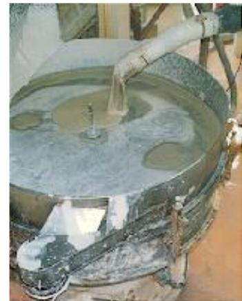
Fig. 4: Clay is passed through a sieve to remove oversized particles. It is then pumped into large storage vats called arks for further processing
