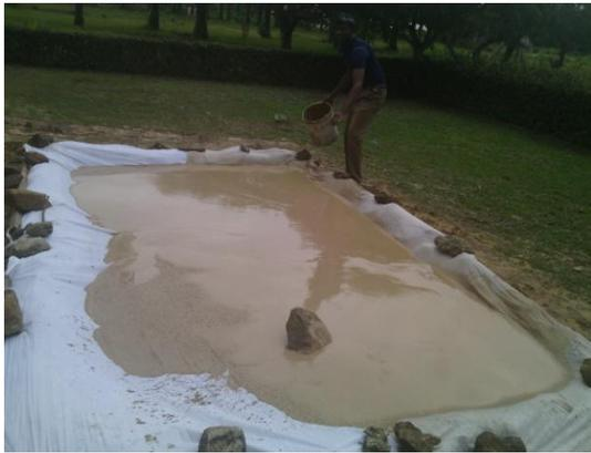
Fig. 9: Pouring clay slip into the trough
