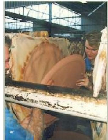
Fig. 6: The time that the slurry remains in the filter press will vary according to the clay body. The moisture content is reduced to about 22%. The clay is removed from the press in the form of cakes weighing 20-45kg
