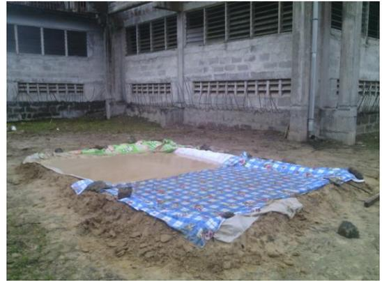
Fig. 10: Half covered clay trough awaiting additional clay slip
