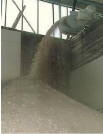
Fig. 1: Raw clay arrives from the quarry and is loaded into a crusher and then conveyed to the storage bins
