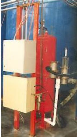
Fig. 5: Pumps and network of pipes feed the slurry into high pressure filter presses
