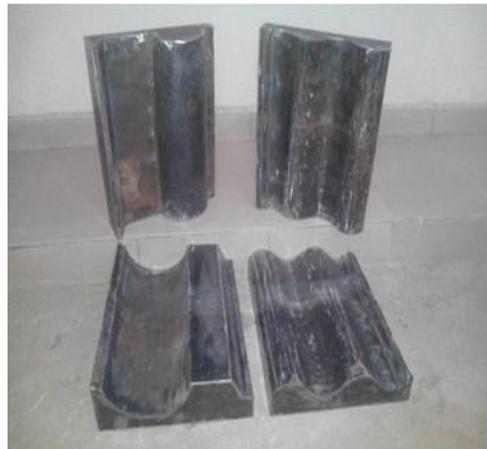
Plate V: Finished (negative & positive) tile mould
