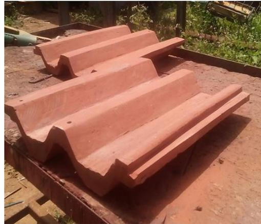
Plate IX: Other samples of fired roofing tiles
