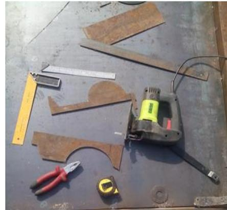
Plate III: Materials used in mould production
