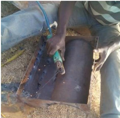
Plate IV: Welding and reinforcement of mould
