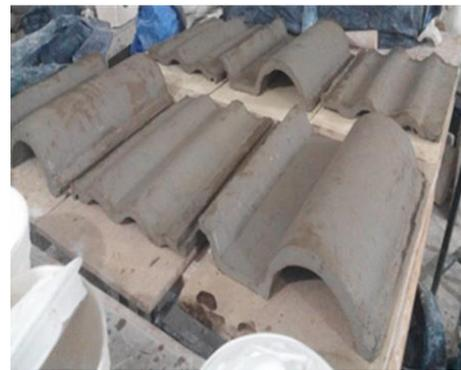
Plate VII: Pressed roofing tiles ready for drying
