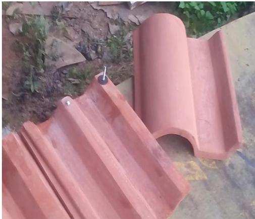
Plate VIII: Fired roofing tiles
