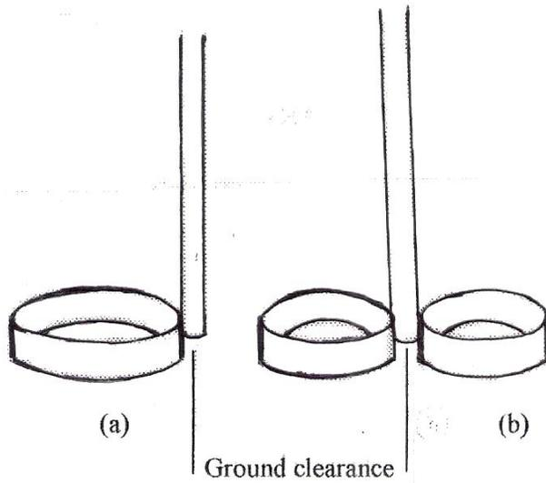
Figs 2 a and b. One and two – chamber metal clay cutters
