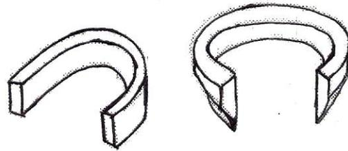
Figs. 3a & b: Unsharpened and sharpened cutting surfaces
