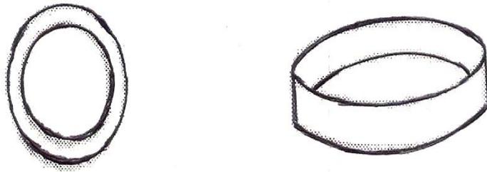
Figs 1a & b. Typical rings sawn out of round pipes
