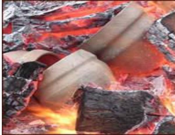
**Plate 2: Open firing process of Ceramic wares by traditional potters**
