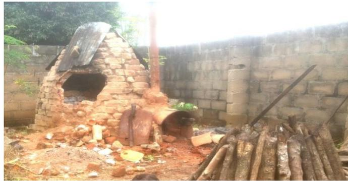
**Plate 3: A local ceramic kiln that uses wood in firing of Ceramic wares by traditional potters**
