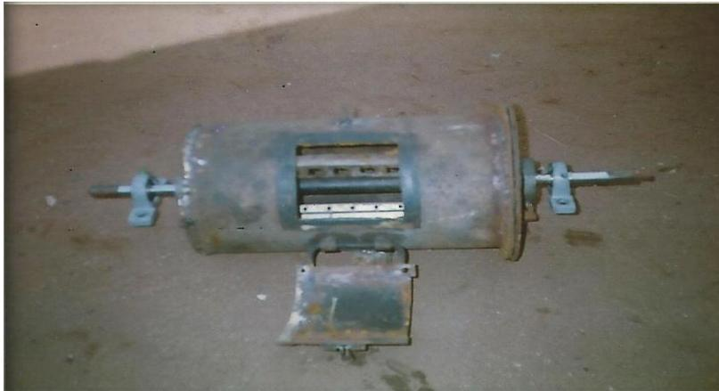
**Plate 6: The tank with two industrial bearings fixed on each side of the shaft.**
