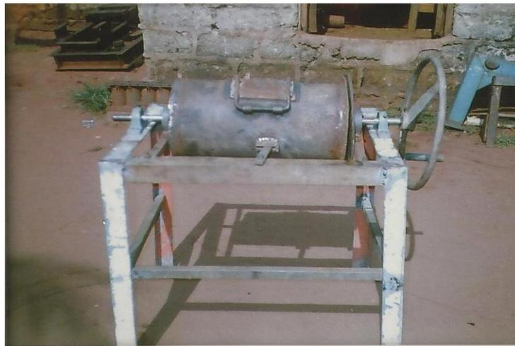
**Plate 8. The complete ball mill.**
