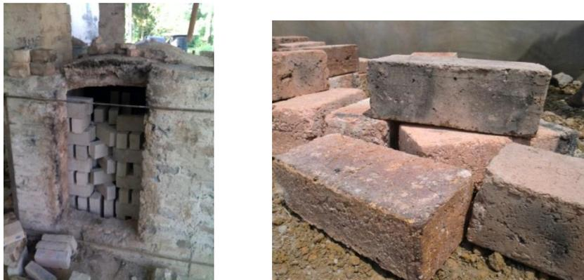
Figure 7: The bricks before and after firing (Photograph by Oluwafemi Adelabu)
