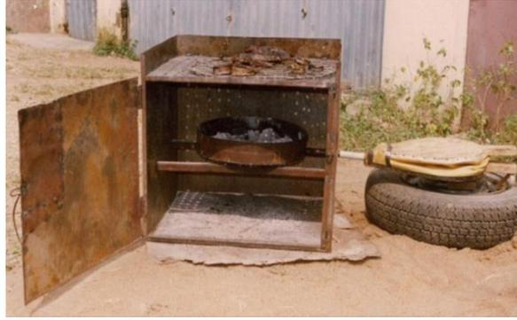
Figure 4: A fish smoking kiln developed by Ikenweuwe N. B., Bolaji B. O. and Bolaji G.A. using galvanized iron sheet and frame. Source: Ikenweuwe et al. (2011)
