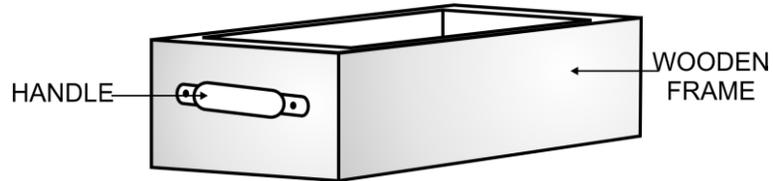
Figure 6: A wooden frame used brick moulding (Adelabu et al. 2007)
