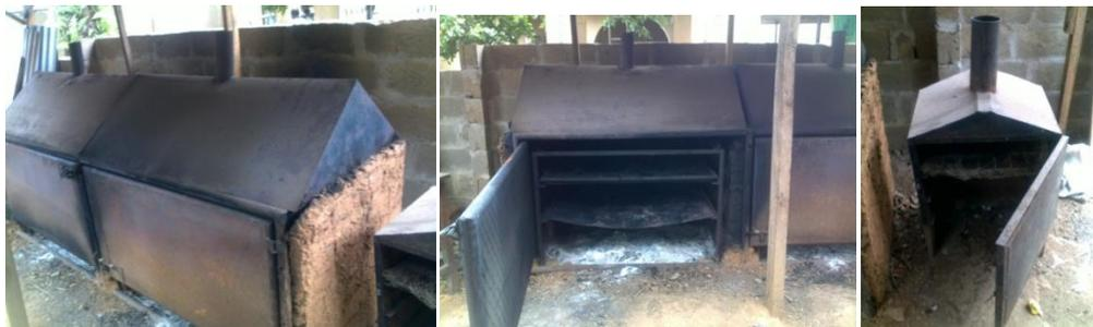
Figure 3: Enclosed smoking kilns developed by Bello M. O. using mud bricks and iron sheet
