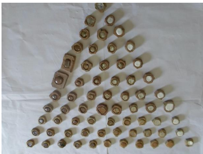
Plate I: Triaxial Blend Result of 66 Samples using Clay, Feldspar, and Quartz
