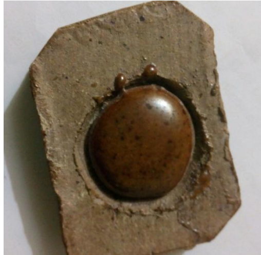
Plate IV: Fired Result of 50% of Majeroku Feldspar and 50% of Ilesa Clay.
