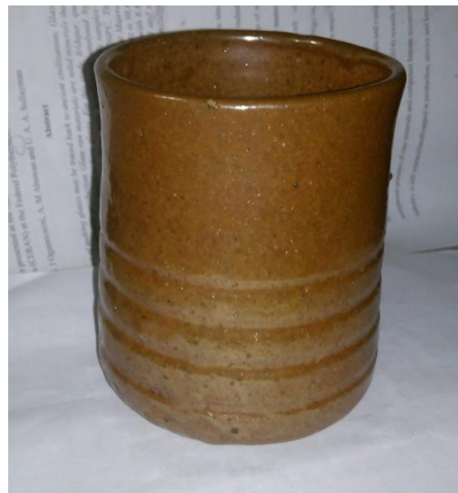
Plate V: Fired Result of 50% Majeroku Feldspar and 50% Ilesa Clay on Stoneware body
