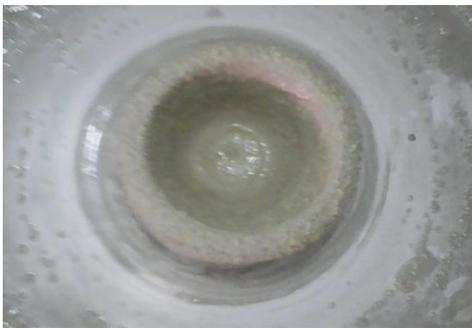
Plate 3: Poor throwing property of body 4 & 5 due to insufficient plasticity
