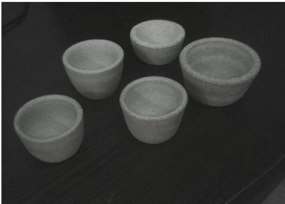
Plates 10: Result of water quenching test of bodies 1-5
