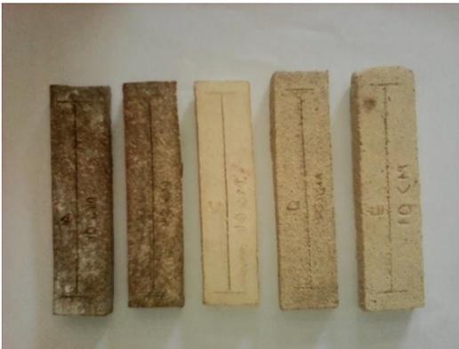
Plate 5: Firing shrinkage bars for bodies 1-5 (A, B, C, D, & E)
