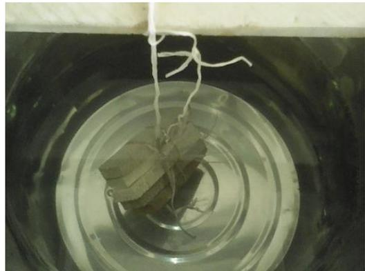
Plate 6: Water absorption test for bodies 1-5 for 2hrs cooled for 4hrs
