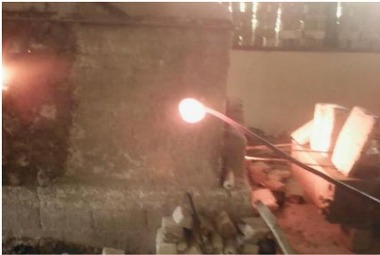
Plate 7: Water quenching of crucible fired to 1300°C during thermal shock resistance test
