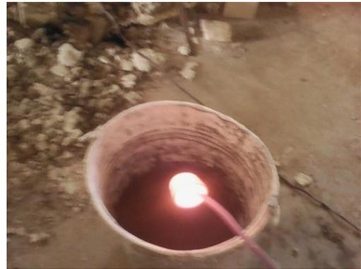
Plate 8: Water quenching of crucible fired to 1300°C during thermal shock resistance test
