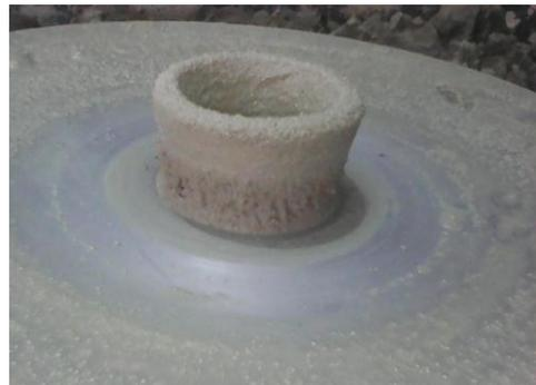
Plate 4: Poor throwing property of body 4 & 5 due to insufficient plasticity
