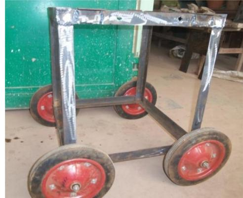
Fig. 8: Detachable pedestal fitted with tyres
