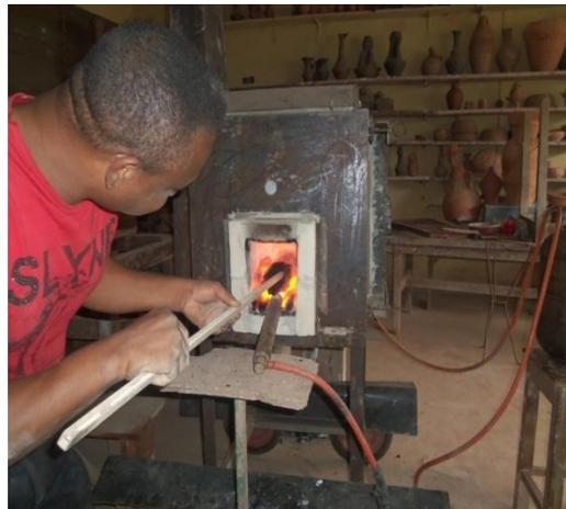
Fig. 14: Test firing the kiln
