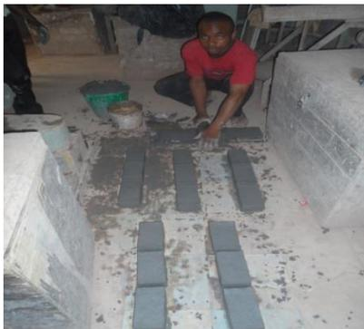
Fig. 3: Molding the bricks
