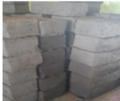
Fig. 4: Molded bricks drying gradually
