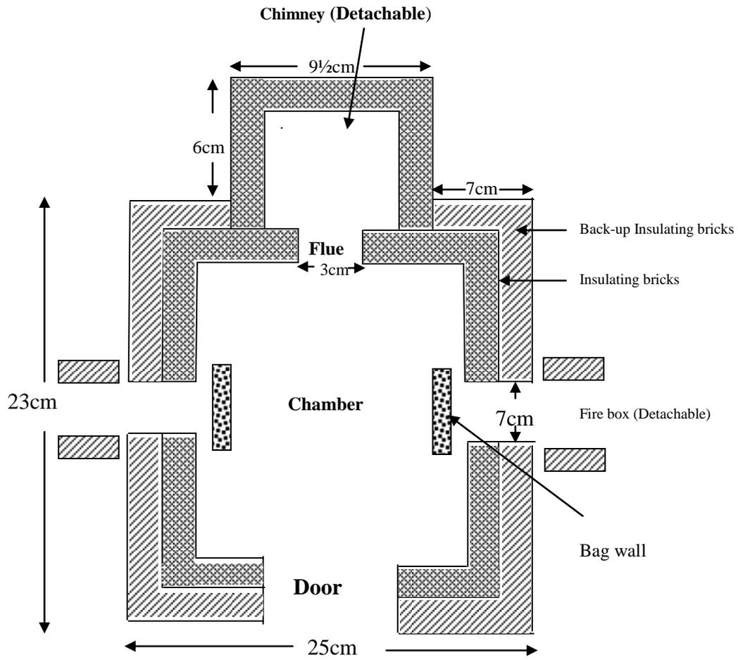
Fig. 5: Kiln plan and dimensions
