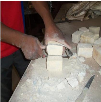
Fig. 10: Cutting the bricks
