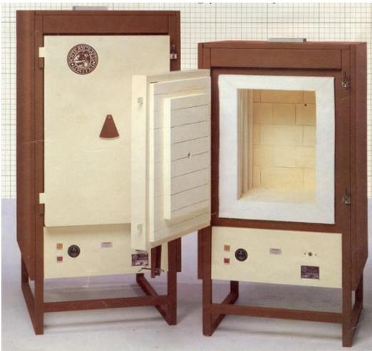
Figure 3: An Electric kiln
